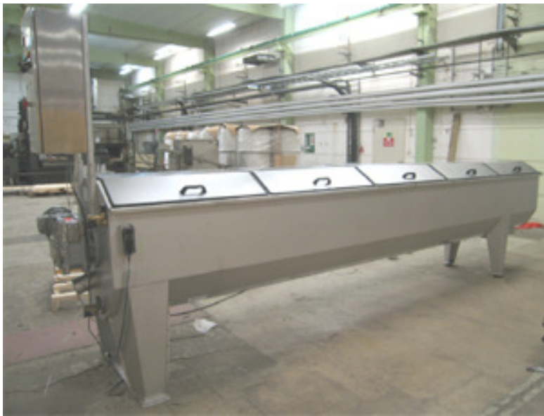
1 pc. Drum thickener Siljan RotoMaster SF35, made of AISI 316L, ready for shipment to a Waste water Treatment Plant in Latvia.
