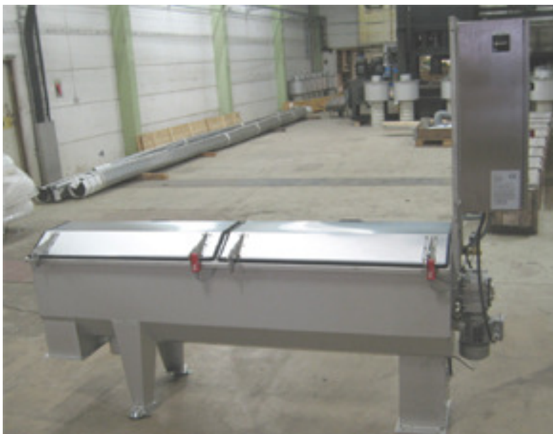
One piece Siljan RotoMaster SF7, including control cabinet and sludge mixing equipment. Ready for shipment to a Waste water Treatment Plant in Romania.
