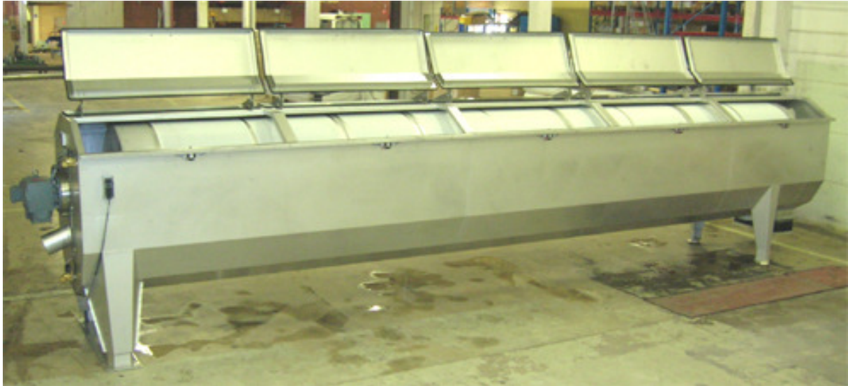
One drum thickener Siljan RotoMaster SF80, Capable of 80 cbm/hour incoming sludge/hour. Ready for shipment to a Waste water Treatment Plant in
