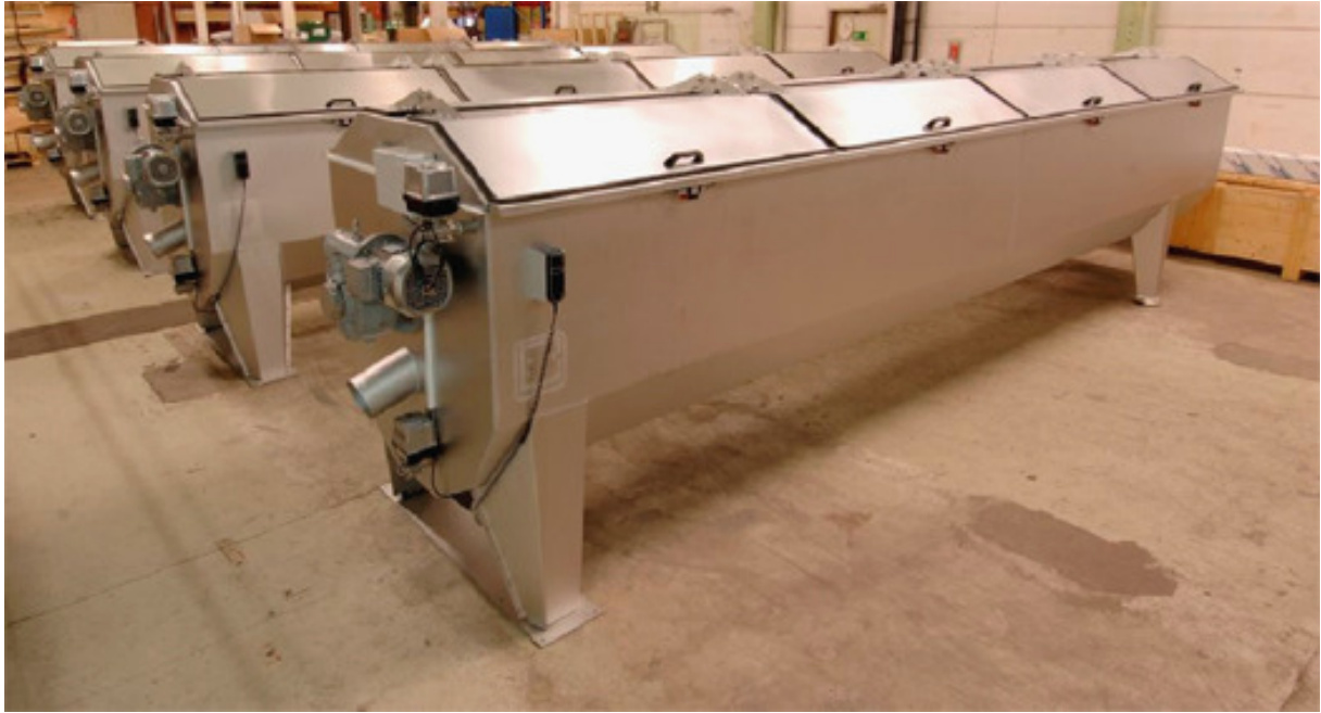
4 pcs Siljan RotoMaster drum thickeners SF60, ready for shipment to a waste water treatment plant in Changsha, PR. of China
