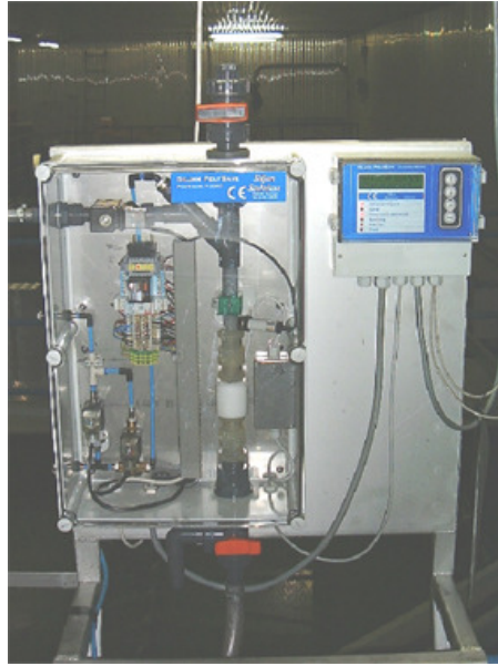
Picture of the control unit Siljan PolySave, with the test unit, including the sensor, to the left and the computer unit to the right.
