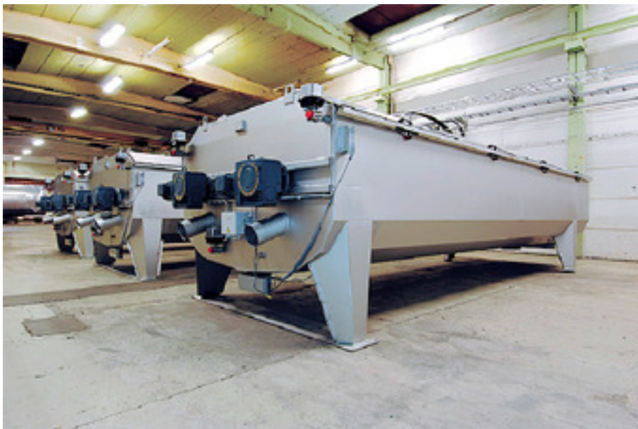
3 pcs. Drum thickeners SF120DUO, capacity of 120 cbm sludge/hour. Ready for shipment to a Waste water treatment plant in Changsha, China.
