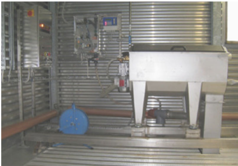
One drum thickener Siljan RotoMaster SF80, Capable of 80 cbm/hour incoming sludge/hour. Ready for shipment to a Waste water Treatment Plant in
